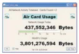
**February**: Air Cards are extremely popular these days especially with the advent of Netbooks. They combine the features of a Wireless Network Card and a Modem to communicate directly from PC to Cell Phone Tower. They provide Internet access, browsing, and file transfer without the normal land-based Internet provider. They can be built into the laptop or pluged-in via a USB or PCMCIA port.
