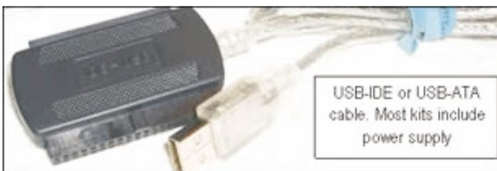
After the bootable CD is created, Power off the computer, then connect the cable to the computer, and the new drive. Put on your good glasses, and examine the large end of the cable closely. There is a set of holes that match the pins on the disk drive, and where is one pin missing on the drive, there is one hole that is plugged on the adapter. If you have an adapter for
