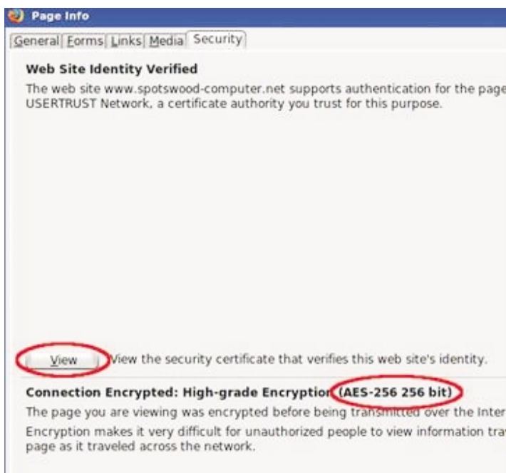
Figure 2: Click on view to see the names. Notice this certificate uses 256 bit encryption.
